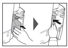
Insert the new waste toner box as shown in the figure. When the box is set correctly, it will snap into place.
